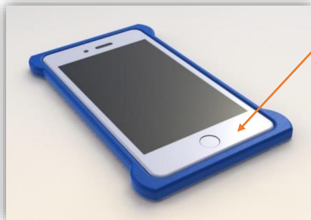
Primary Cell- phone Antenna Area
